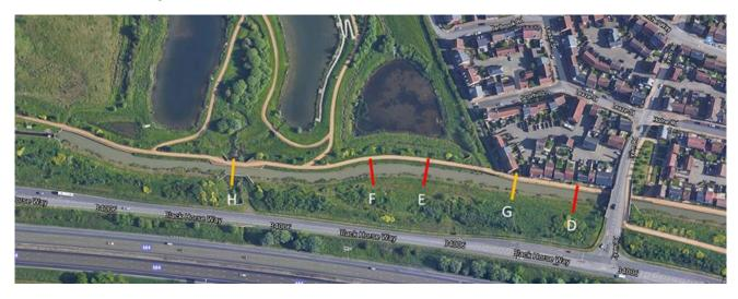
A series of test pits were therefore dug both sides of the canal and monitored to see if they would fill with water. This would indicate whether water was passing through the banks of the canal, and if so where.
