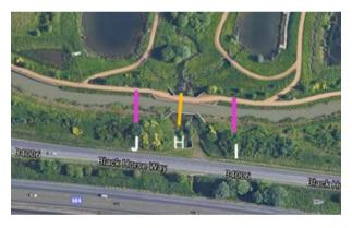
It has therefore been concluded further works to the northern bank are required, with the steel sheet piles sealed from within the canal. The same fixes will also be applied to the western section J to H.
