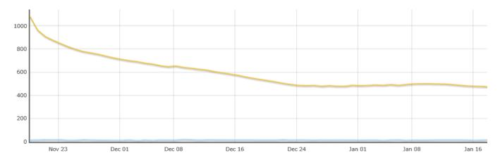
These readings provide positive evidence that the main leak in the base of the canal has been fixed. The water is however still dropping at a faster rate than either of the adjoining sections.
